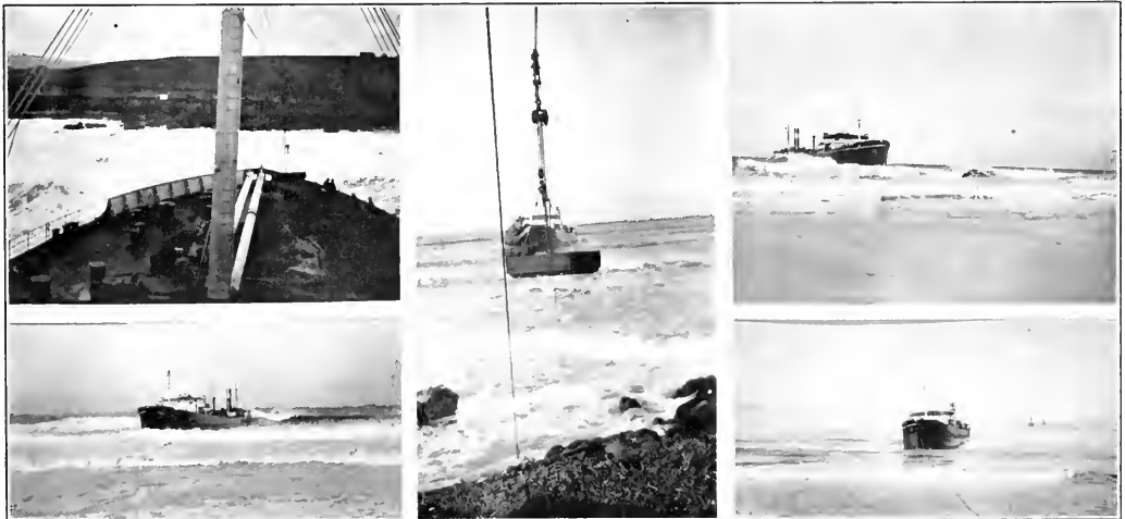
Some views showing the tanker Tamiagua in the surf near Pescadero Point and the high line which was used, on account of the heavy sea, to convey materials for salvage to the stranded vessel.
